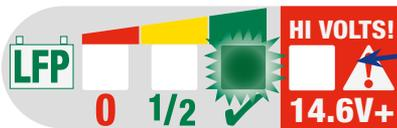
Confirms higher charge status of LiFePO<sub>4</sub> battery
